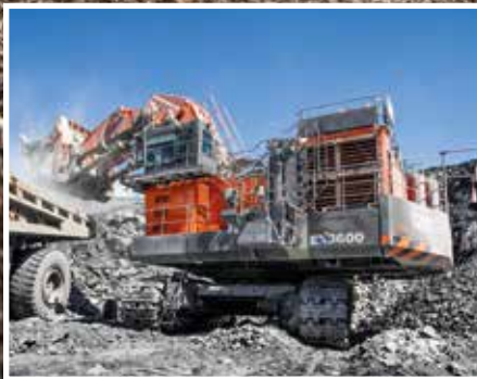
EX ultra-large excavators
