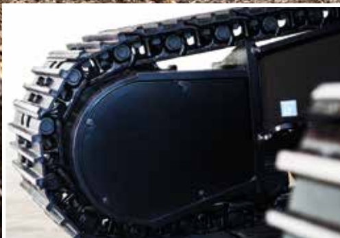
A thicker travel motor cover offers greater protection against damage.
